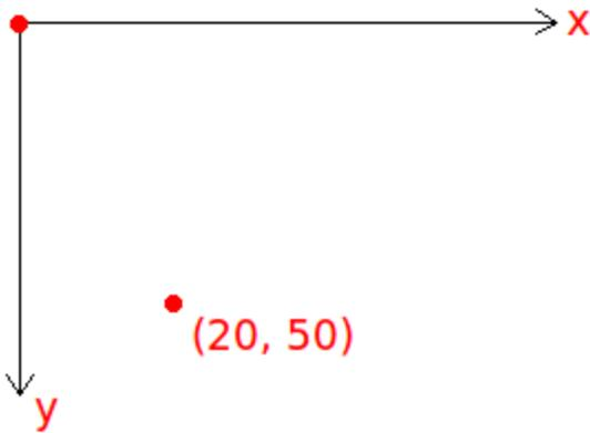
In this quick sketch I made it's easy to understand how coordinates work on wxPaintDC.
