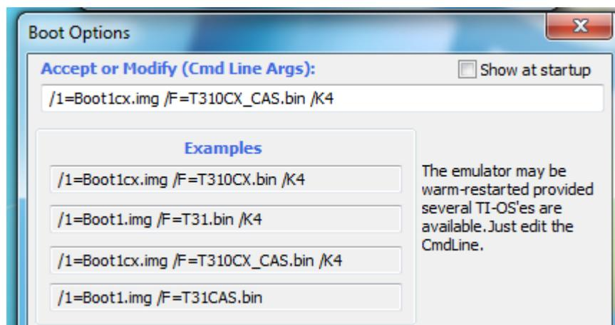
Uncheck the checkbox 'show at startup' and Press OK. This time the booting up process should be much faster. Because we have selected the touchpad keypad (/K4), you should get something like what is shown in the following picture.
