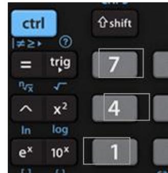
b. As you can see above, the keys are misaligned. Press Ctrl+A (Edit->Arrange keys). Draw a drag rectangle around these keys. The 'green' is the first in the selection (the alignment reference) and the 'blue' is the 'last'.
