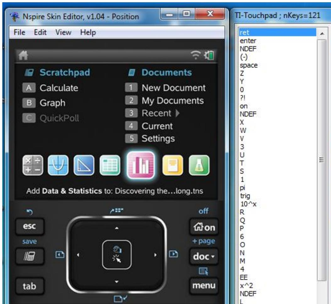
a. Define the key position: using the mouse (LeftButton) draw a drag-rectangle around the key 'ret'. You'll see a rect-tracker over the top (in red) to let you adjust the size and the position.
